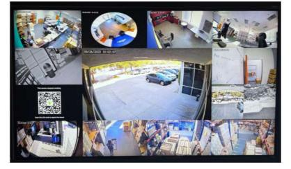
remote management interface. Admins can configure grid layouts for all their CamViewers remotely. The device will then operate like a local system, connect to the cameras, and show local video streams at up to 30 FPS for up to 24 simultaneous video feeds.
